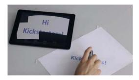
PocketScan performs character recognition for 130 languages. The device measures  $95 \times 50 \times 27$  mm (3.75 x 2 x 1 inches), weighs 85g (3 ounces) and can scan 400 times between charges. The cheapest PocketScan will cost \$99 for Kickstarter users who pay in advance, a \$50 discount from the anticipated retail price. The producing company hopes to ship it in December. Competitors include NeatReceipts and ScanSnap.
